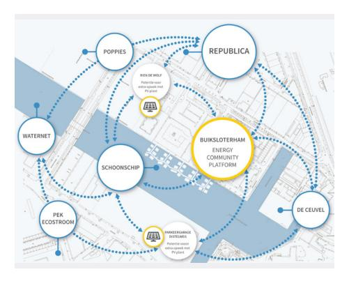
Over the last couple of years, the innovation company Spectral has been working with energy communities and project developers to realise smart microgrids in the Buiksloterham neighborhood in Amsterdam north. Within the ATELIER project, these smart microgrids will be integrated into an overarching, district-level smart-grid in order to increase the benefits to the communities, better balance the local energy supply and demand, and integrate even more renewables.
